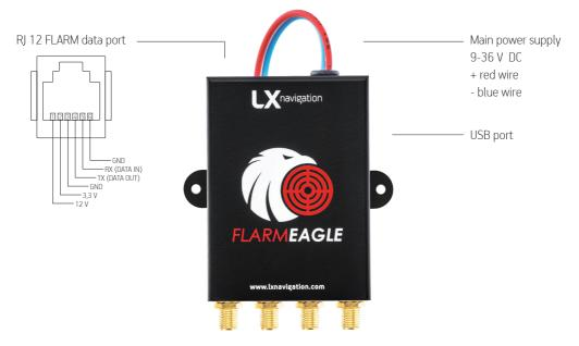
SMA connectors are marked with antenna type
